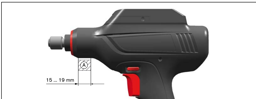
Fig. 4-7: Torque support clamping area
