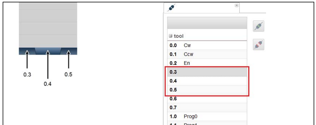
Fig. 3-3: Function fields for program selector in center position.
